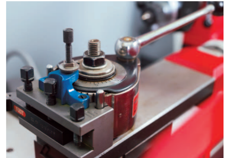
Fast-change tool holder. To speed up the machining process, there are several tool holding systems available. This ensures that tools can be changed quickly.
