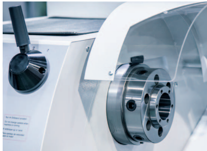
Safety. For the safety of the operator, the chuck protection and wheel caps are monitored by an electric switch.
